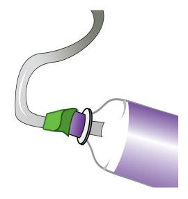
Place one end of the tubing into an empty 2-liter bottle. Using duct tape (or masking tape if held tight), connect the tube to the bottle opening creating an air-tight seal.
