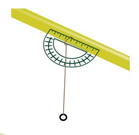
Tie a string to the center hole of a protractor and connect the large paper clip (a washer or nut can be substituted) to the other end of the string so that it acts as a weight. Tape the protractor to the center of the PVC pipe and allow the string to hang freely. This will allow learners to measure the launch angle.
