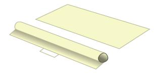
Cut an 8  $\frac{1}{2}$  x 11 in. piece of scrap paper in half, creating two 8  $\frac{1}{2}$  x 5  $\frac{1}{2}$  in. pieces. Wrap one of the pieces of paper around the PVC pipe, and tape into a tube shape. The tube should fit snugly but be able to slide over the end of the PVC pipe.
