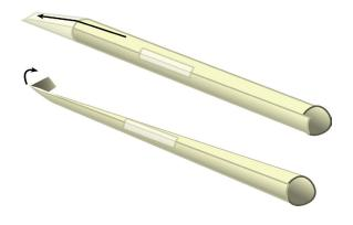
Fold the end of the paper tube and fasten with tape to seal it.
