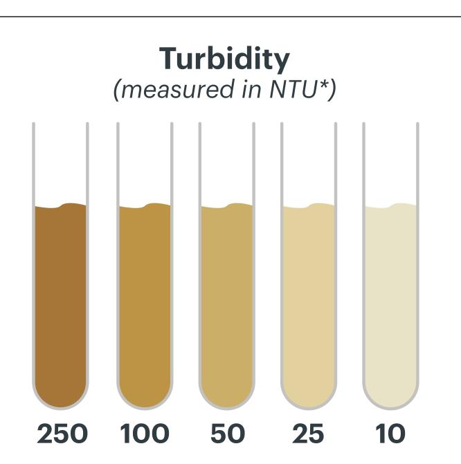
\*NTU: Nephelometric Turbidity Units, measure the intensity of light scattered at 90 degrees as a beam of light passes through a water sample.
